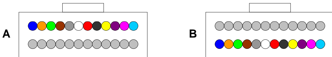
Figure A6: Key-up/Key-down Patchcords Mirror Signals About the Horizontal Axis
