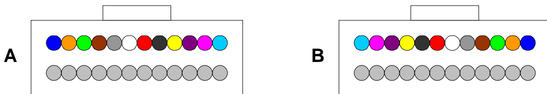
Figure A3: Key-up/Key-up Patchcords Do Not Mirror About the Horizontal Axis
